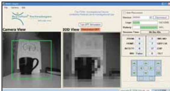
Figure 3. Training performance is monitored using an accessory that displays video from the user mounted camera (top) and provides a visual depiction of the stimulation pattern on the tongue (bottom).
