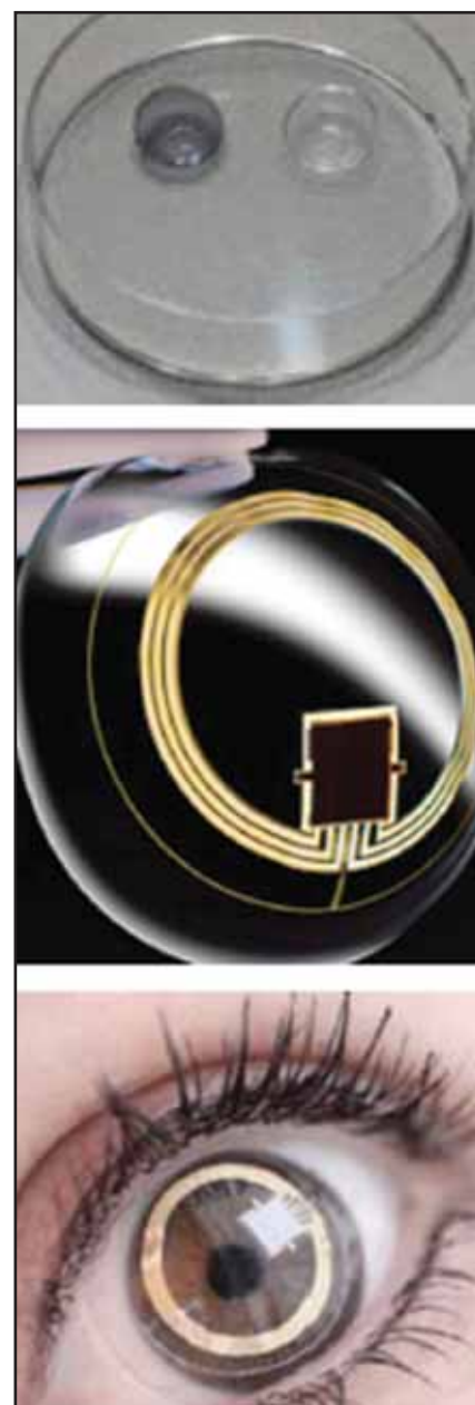
Figure 4. (Top) Prototype photochromic contact lens; (center and bottom) Triggerfish lens for continuous IOP measurement.
