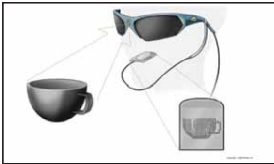
Figure 3. Training performance is monitored using an accessory that displays video from the user mounted camera (top) and provides a visual depiction of the stimulation pattern on the tongue (bottom).
